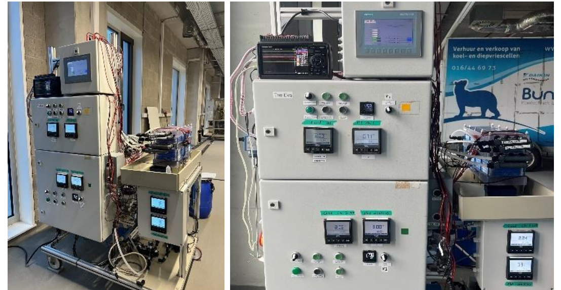
Electrodialysis to remove salts
